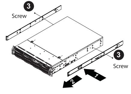
Figure 8: Attaching the rails to the chassis.
